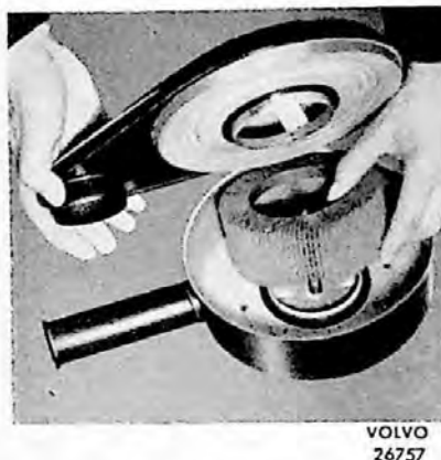
Fig. 15. Replacing the filter insert (B 18 A).
