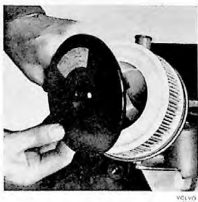
Fig. 14. Replacing the filter insert (B 18 D, right-hand drive).
