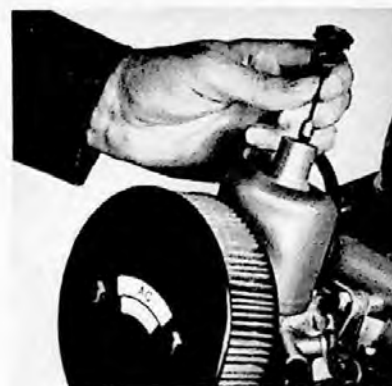
Fig. 2. Checking the oil level.
