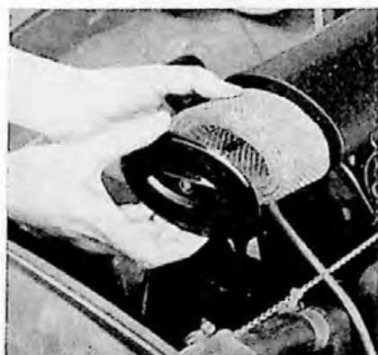
Fig. 11. Removing the filter element (B 16 A).
