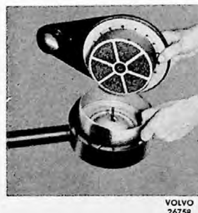
Fig. 17. Disassembling the air cleaner (B 18 A, B 16 A).
