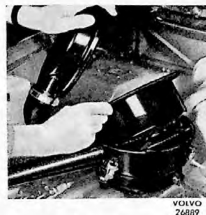
Fig. 16. Disassembling the air cleaner (B 18 B, B 18 D).
